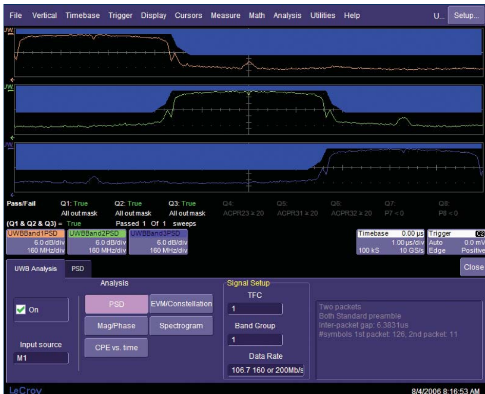
Power Spectral Density (PSD) mask testing performed simultaneously in TFI mode.
