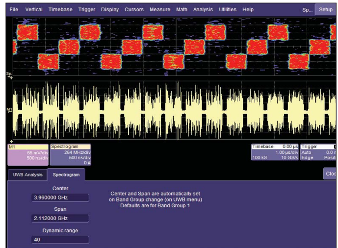
Spectrogram of a UWB signal hopping over three frequency bands of a band group
