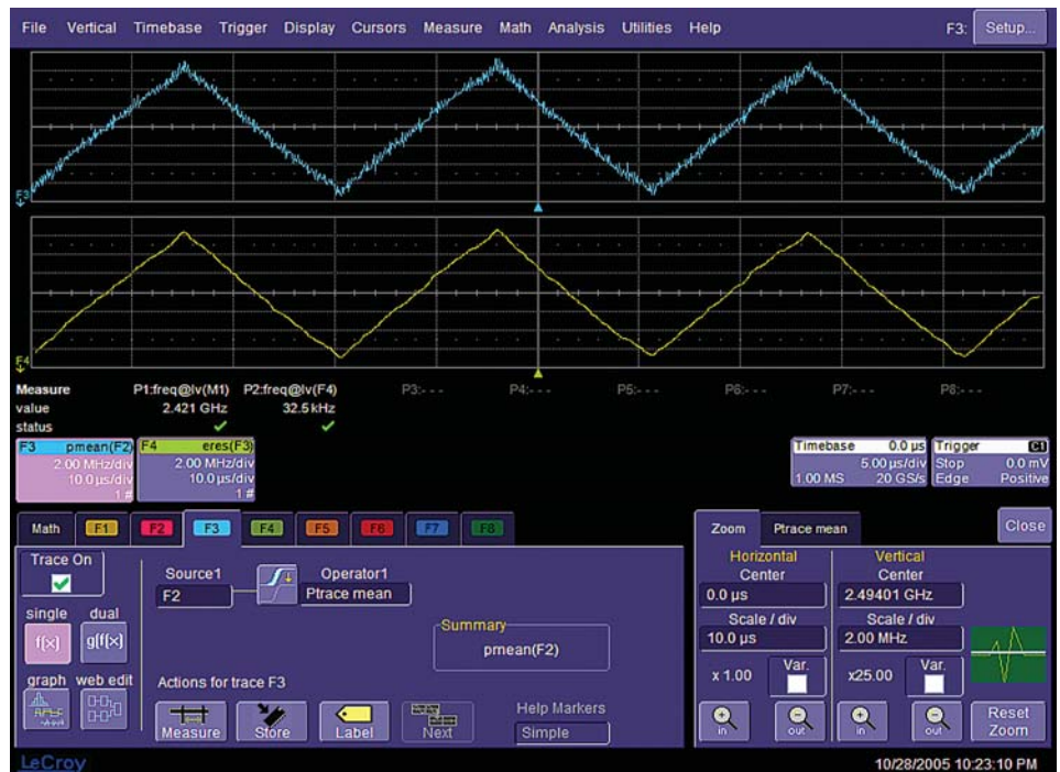
See multiple cycles of spread spectrum clocking.
