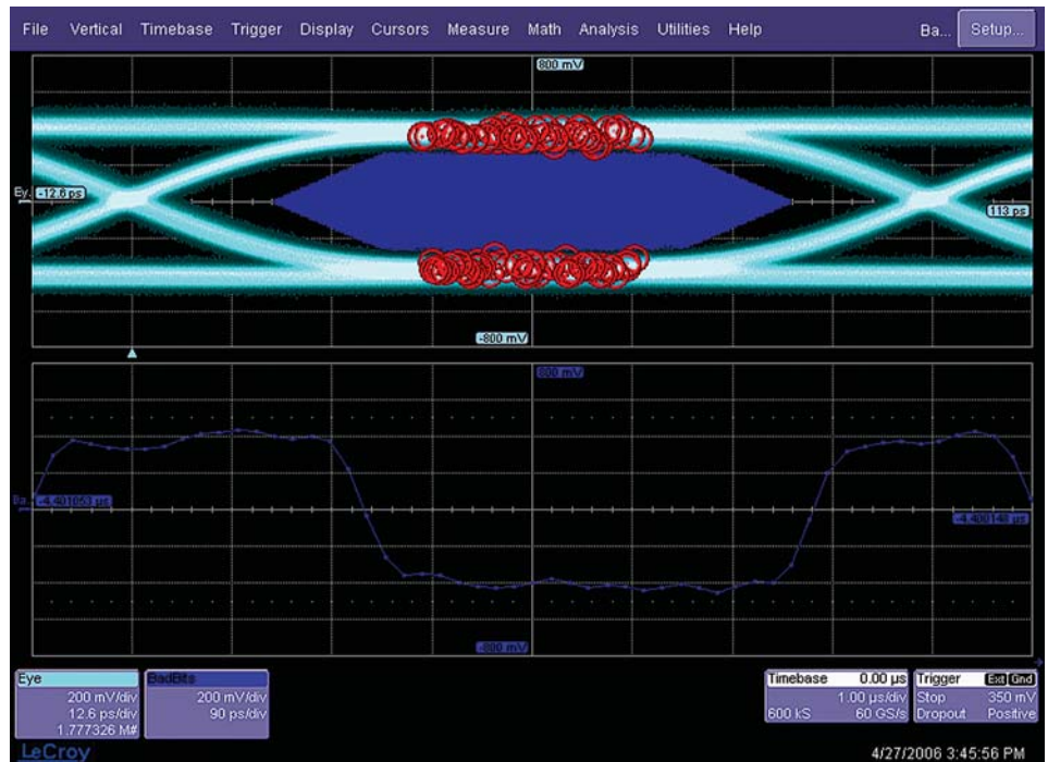
Observe bit sequences that cause mask violations.
