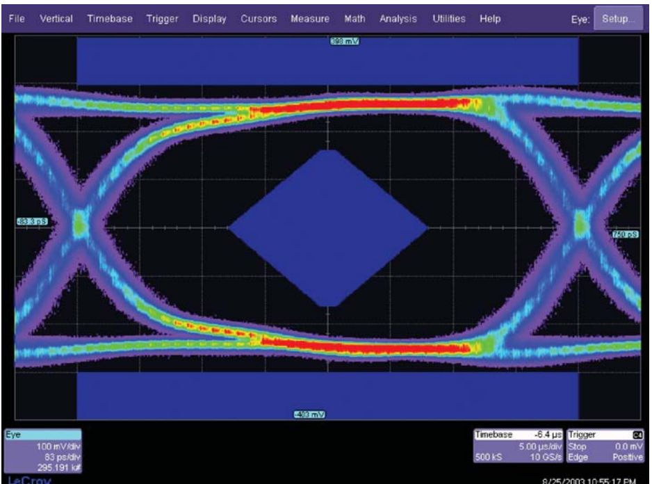
Eye pattern of serial ATA signal.
